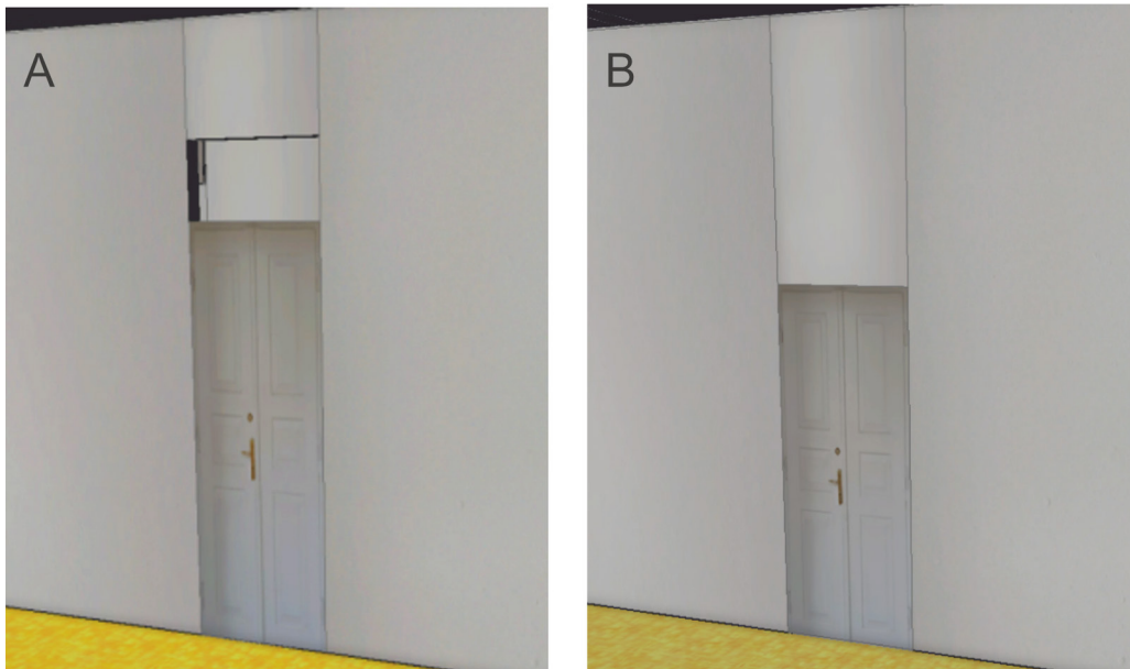
Fig. 2. Correction of the door height: A) before the change, B) after the change
