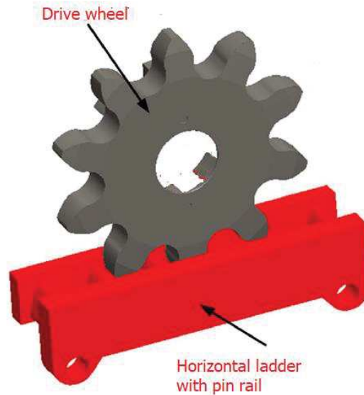
Fig. 12. Eicotrack chainless haulage system– general idea [11].
