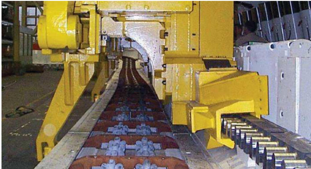
Fig. 4. The Saartrack chainless haulage system [7]
