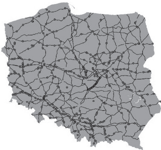
Fig. 2. Weather stations coverage on national roads in Poland [own study based on GDDKiA data]
