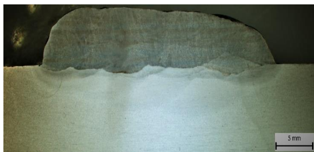
Fig. 3 Welding macrostructure OK 55 T
