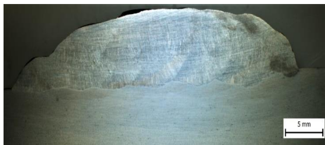
Fig. 2 Welding macrostructure OK 50 T
