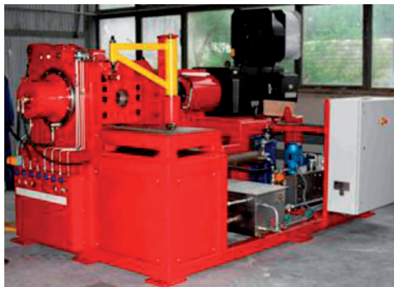
Fig. 4. View of the MC-260 device for continuous rotary extrusion made by Meltech-Conflex Limited operating at IMN-OML
