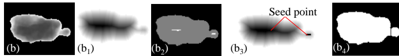
(ii) Number of connected domains of the second MGTS is 0. (b) Grayscale map without background; (b 1 ) Distance map; (b 2 ) Distance transformation to calculate seed point; (b 3 ) Water injection to find ridge line. (b 4 ) Segmentation result
