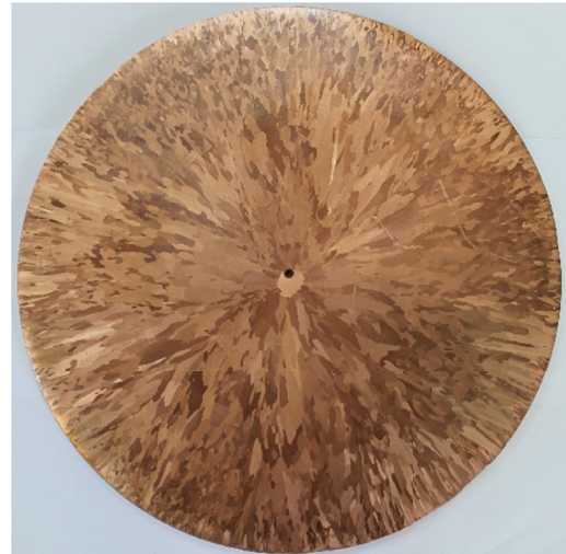
Fig. 2a. Morphology of the continuously cast brass ingot revealing columnar (dominant), equiaxed grains and the single crystal situated axially.
