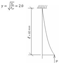
2. Sewing needle with a constant (CSA) average value i.e. I' = constant (axial load is concentrated)
