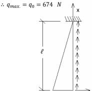
6. Axial load is parabolic (left-hand)
