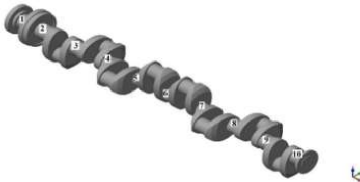
Fig. 4 Modeled medium speed crankshaft of the Buckau Wolf R8DV 136 main drive
