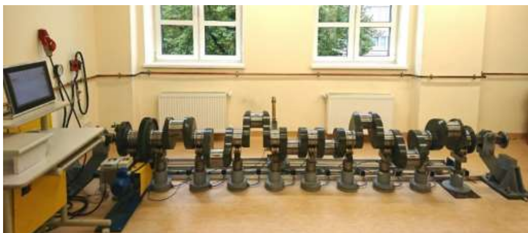
Fig. 1 The prototype test rig developed at the Maritime University of Szczecin for measuring geometrical deviations of large crankshafts with a flexible support system
