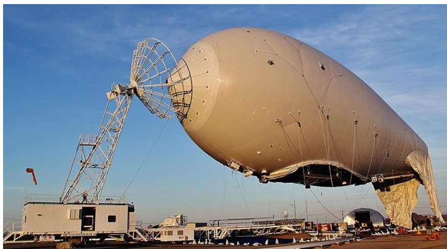
Rys. 5. Tethered Aerostat Radar System [21]
