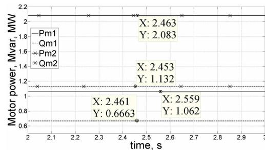
Fig. 3. Active and reactive power consumed by M1 and M2 at rated load  $P_{M1} = 1.062$  MW,  $Q_{M1} = 0.6663$  Mvar,  $\cos\phi_{M1} = 0.847$ ;  $P_{M2} = 2.083$  MW,  $Q_{M2} = 1.132$  Mvar,  $\cos\phi_{M2} = 0.879$
