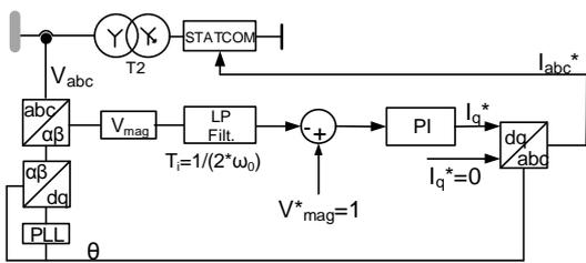
Fig. 1. Control structure used for STATCOM voltage regulation
