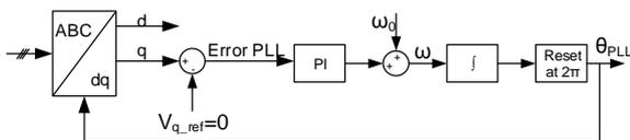
Fig. 2. Phase-Locked Loop
