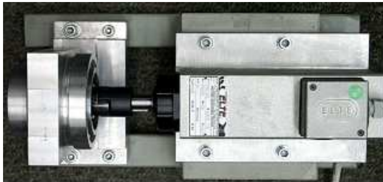
Figure 5: Photo of the pumping engine with a Roto-Jet pump of the PCz 95.7 type [26].
