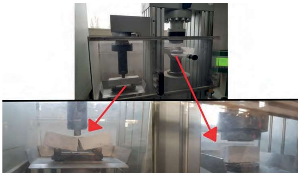
Fig. 4. Laboratory testing of proposed mixtures; left – measurement of flexural strength, right – measurement of compressive strength
