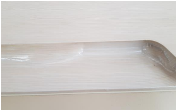
Fig. 1. The unstretched foil on the furniture front
