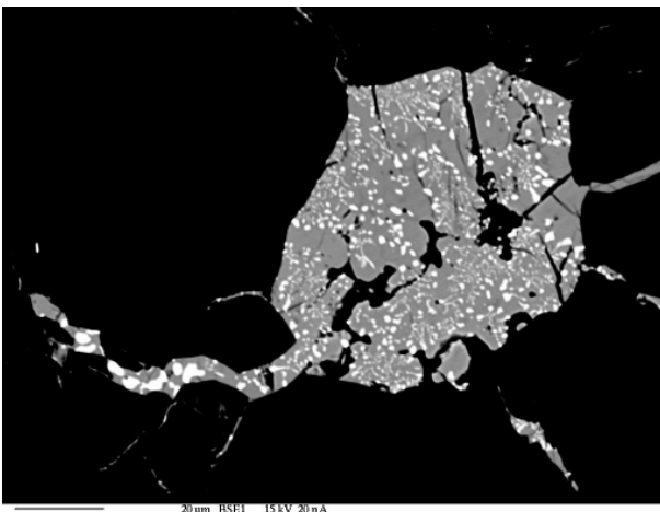
Fig. 9. Minor FeNi-metal within a grain of troilite. SEM (BSE image)
