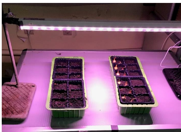
Photo 1. The appearance of the stand for the study of bioefficiency of fertilizers introduced into magnetized technogenic soils (phot. S. Kovshov)
