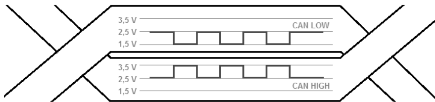
Fig. 1. Signal transmission in the CAN twisted pair [9, 10]
