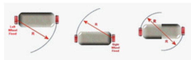
Fig. 6. Visualizing the spatial relationships in pivoting around one stopped wheel or around the robot center
