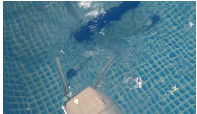
Fig. 13. The position of the mini CyberSeal tail fins during maneuver of turning left
