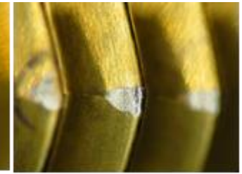
Fig. 14. The new and worn forming lobes
