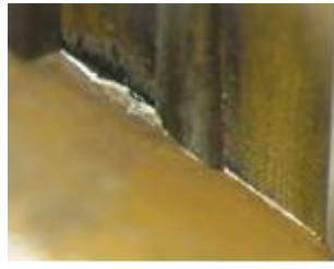
Fig. 13. The new and worn cutting edge
