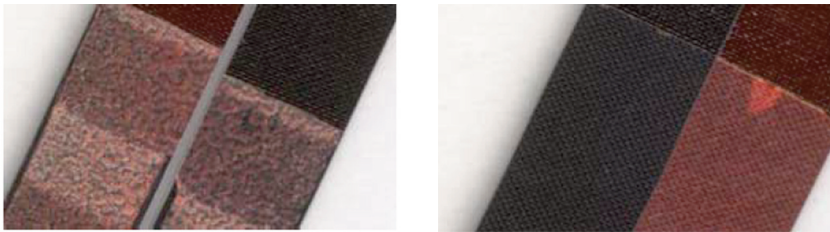
Fig. 8. Cohesive (left) and adhesive (right) failure of bonded joint [16].
