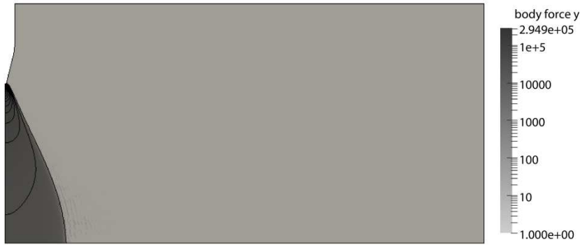
Fig. 6. Distribution of body force y component in \text{N/m}^3 (y axis pointing downwards)
