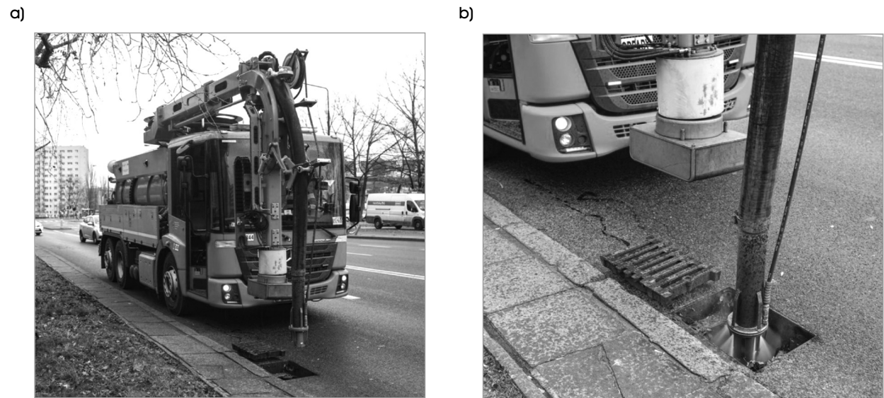
Figure 4 A specialist truck for cleaning the sewage system, FFG Elephant type: (a) general view, (b) sewage collector cleaning
