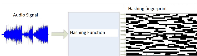
Fig. 2. Signal parametrization using hashing function.
