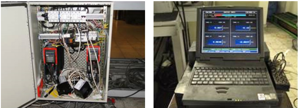
Fig. 4. Testing stand measuring system, control system cabinet at the left side and measurement computer with docking station at the right side
