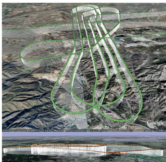
Fig.1. Visualization of postprocessing data (RTK/INS) gathered during the fly over the Mielec airport and GPS/GPRS device for real time monitoring as a second monitoring system on airplane Piper PA-34 Seneca II
