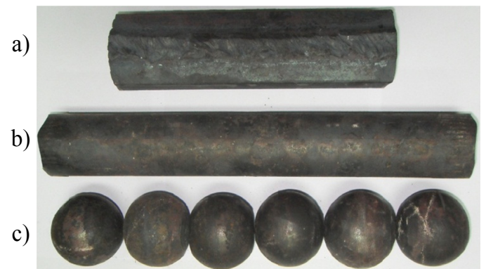
Fig. 7. Semi-finished products and finished products produced using a flat wedge reversing mill: a) railway rail head pre-forged in a hexagonal pass, b) bar formed with the upper tools, c) forgings of balls formed with the lower tools
