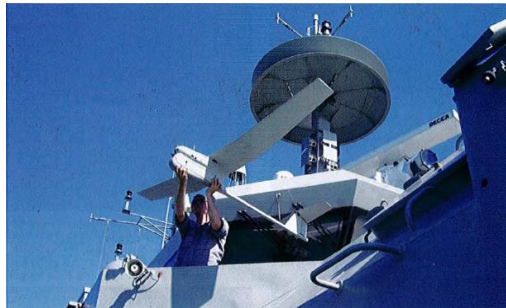
Fig. 1. The launch from a hand of an AQUA PUMA mini-UAV [10]
