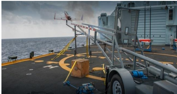
Fig. 6. The launch of a UAV from the launcher mounted on the board of a naval vessel [12]
