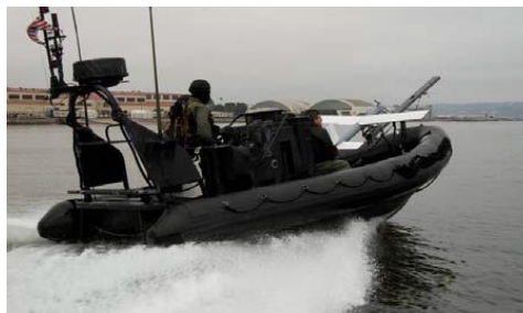
Fig. 5. The launch of a Silver Fox mini-UAV from the board of a USV [7]
