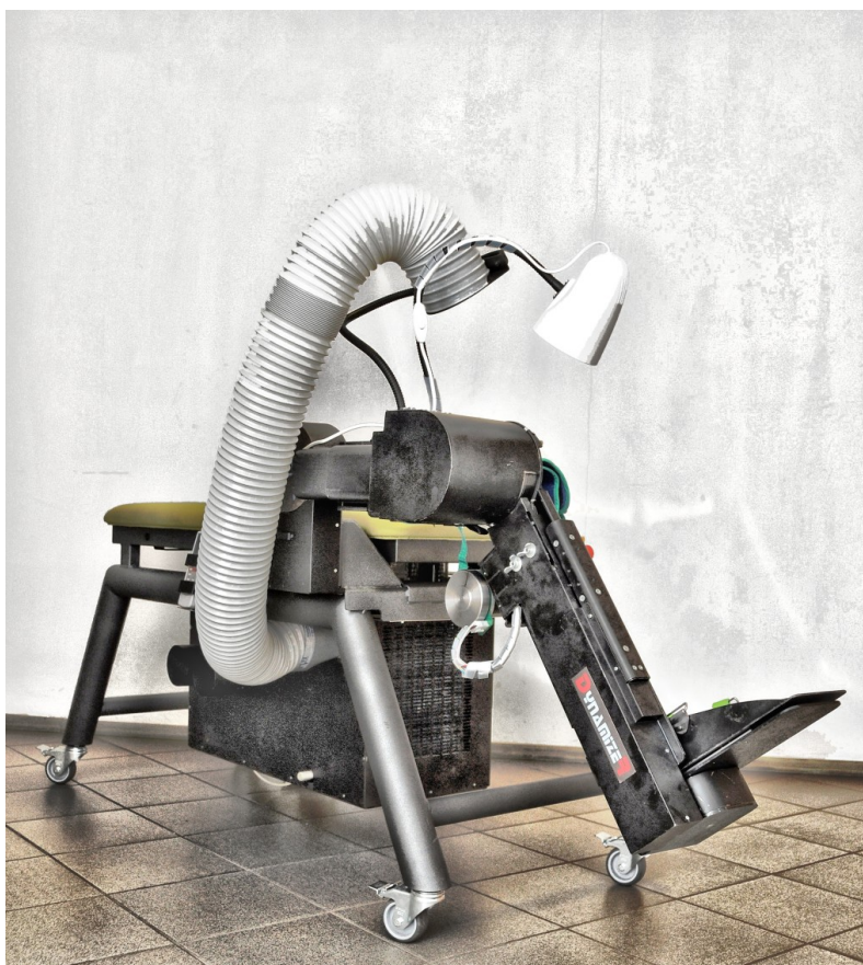
Fig. 1. Dynamizer - a device for knee joint rehabilitation.
