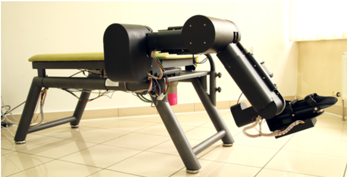
Fig. 2. LEG-100 - device for the lower limb rehabilitation.
