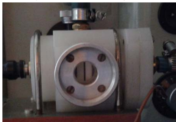
Fig. 2. External view of the discharge chamber.
