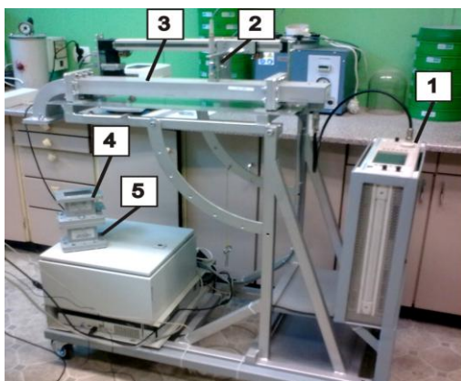
Fig. 1. View of a microwave slot line device: 1 - low power microwave generator ( f = 2.45 \text{ GHz} ), 2 - diode detector, 3 - rectangular waveguide with a slot, 4 - chamber for tested materials, 5 - microwave waveguide damper
