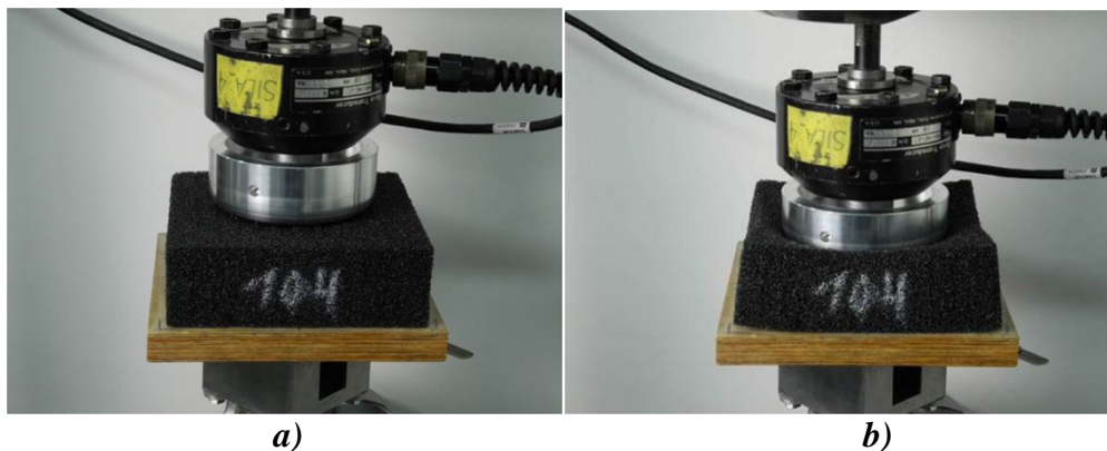
Fig. 2. Indenter and S28280 auxetic foam sample: a) before the test, b) during 40,000 cycle [6]
