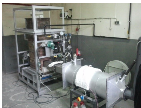
Fig. 1. View of the research stand for the thermal utilisation of post-reclamation dusts: in the stage of testing operations in the final version
