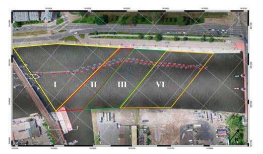
Figure 7. Digital orthophotomap with established trajectories: from the GNSS receiver (blue) and from the CCTV camera (red)
