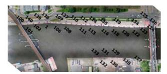
Figure 4. Digital orthophotomap developed on the basis of UAV flights with photopoints measured using a GNSS receiver with RTK correction
