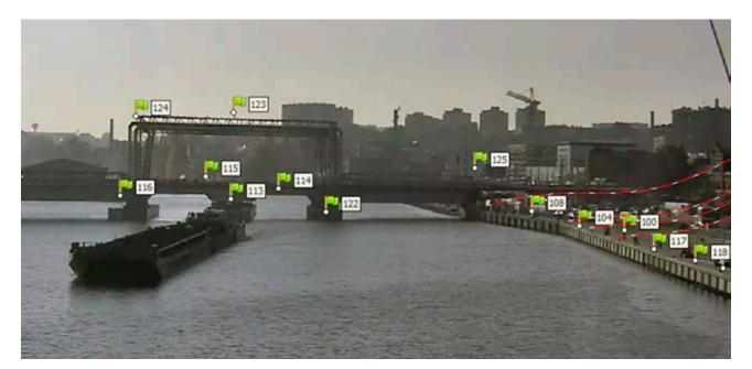
Figure 5. Calibration of the non-metric camera based on the points measured by an electronic tachymeter
