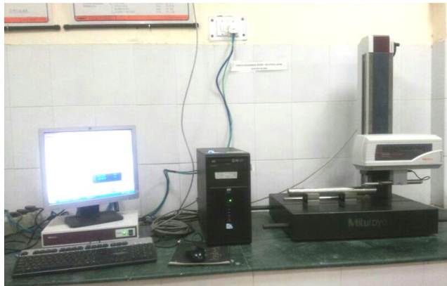
Fig. 2. Photograph of surface roughness measurement test set up
