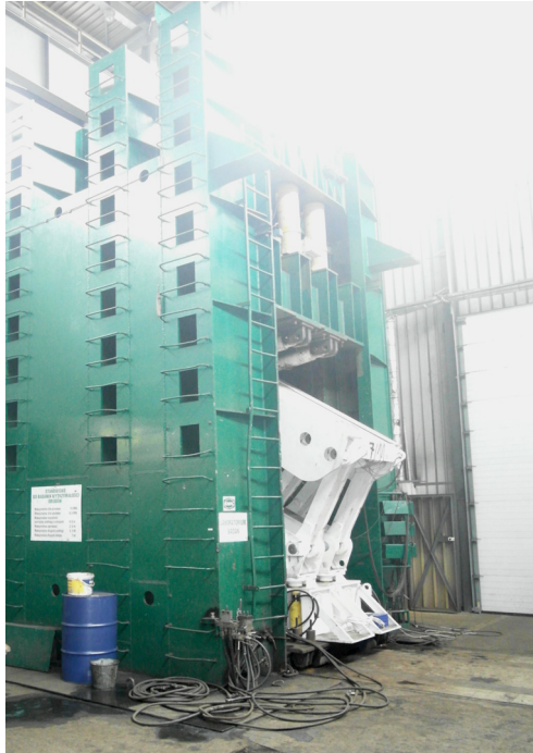
Fig. 4. BW 16/34 POz roof support placed in the test rig and founded on the “hydraulic cushion” at the KOMAG Institute of Mining Technology in Gliwice
