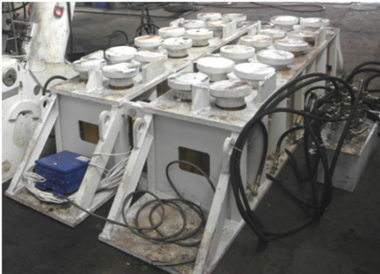
Fig. 5. Hydraulic cushion used during laboratory tests to simulate different values of compression strength of floor rocks and different arrangement of support scheme
