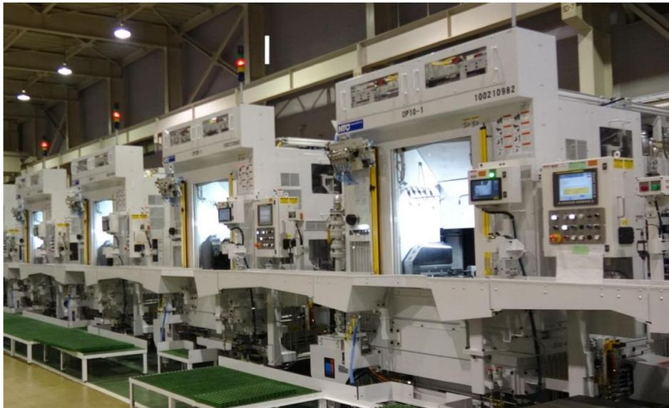
Fig. 12. FTL for cylinder block machining (by courtesy of Komatsu NTC, 2017)
