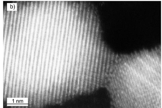
Fig.4. MWCNTs-Re\_4 nanocomposite: a) MWCNTs decorated with Re nanoparticles, BF, HRTEM; b) crystal structure of Re nanoparticles, HAADF, STEM
