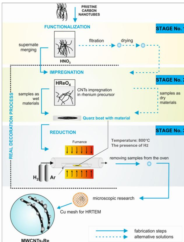
Fig. 1. The process diagram of MWCNTs-Re nanocomposites manufacturing by the high-temperature method (based on [27])
