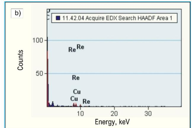
Fig. 5. Cluster of MWCNTs decorated with Re nanoparticles; HAADF, STEM (a); Qualitative analysis of the chemical composition from the area marked with a blue frame in 5a figure, EDS (b)
