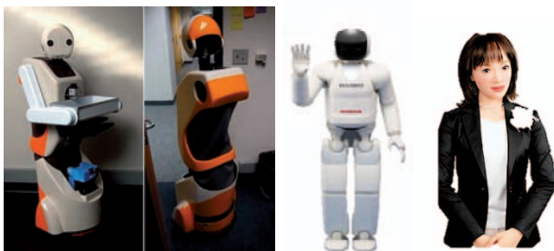
Fig. 2. Robot design, from left to right: Snackbot (machine-like design), Asimo (humanoid design), Actroid DER (android design)
