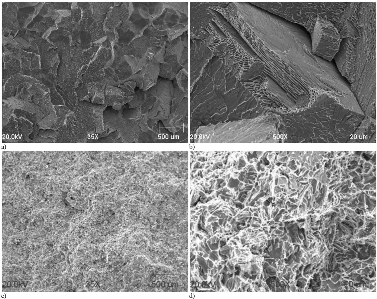
Fig. 5. Microstructure on alloy section as-cast (a, b) and after the spheroidising treatment (c, d); (SEM)
