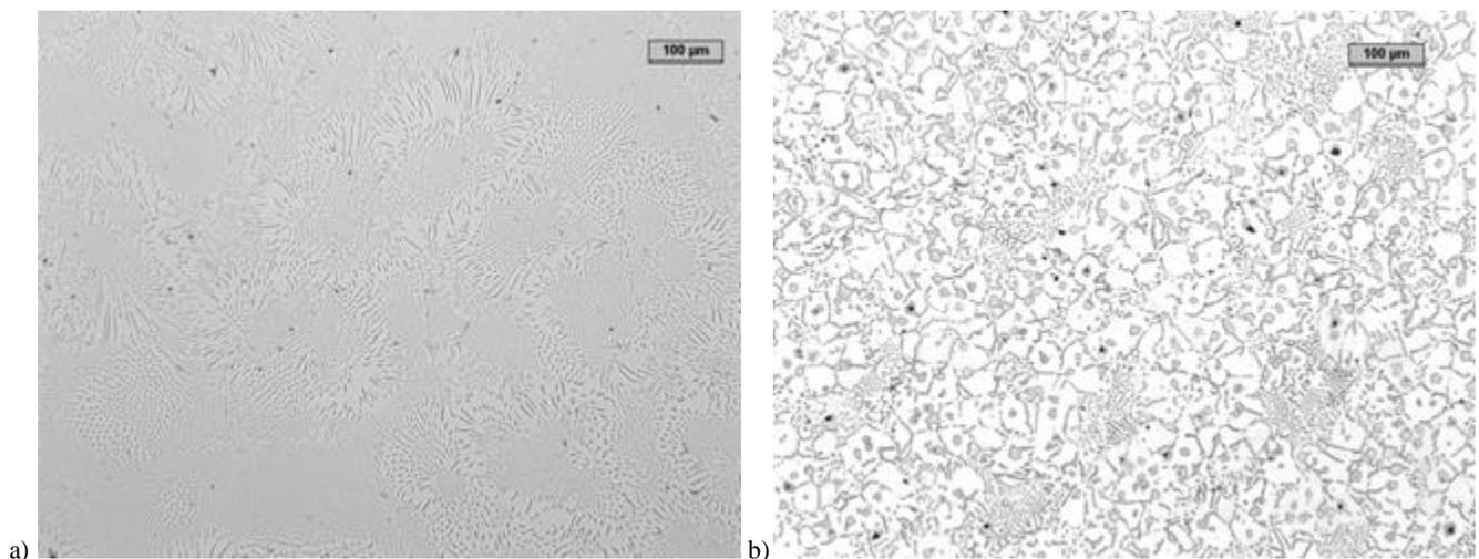
Fig. 1. Microstructure of base alloy (a) and of alloy subjected to spheroidising treatment (b); etched in Vilella's reagent
