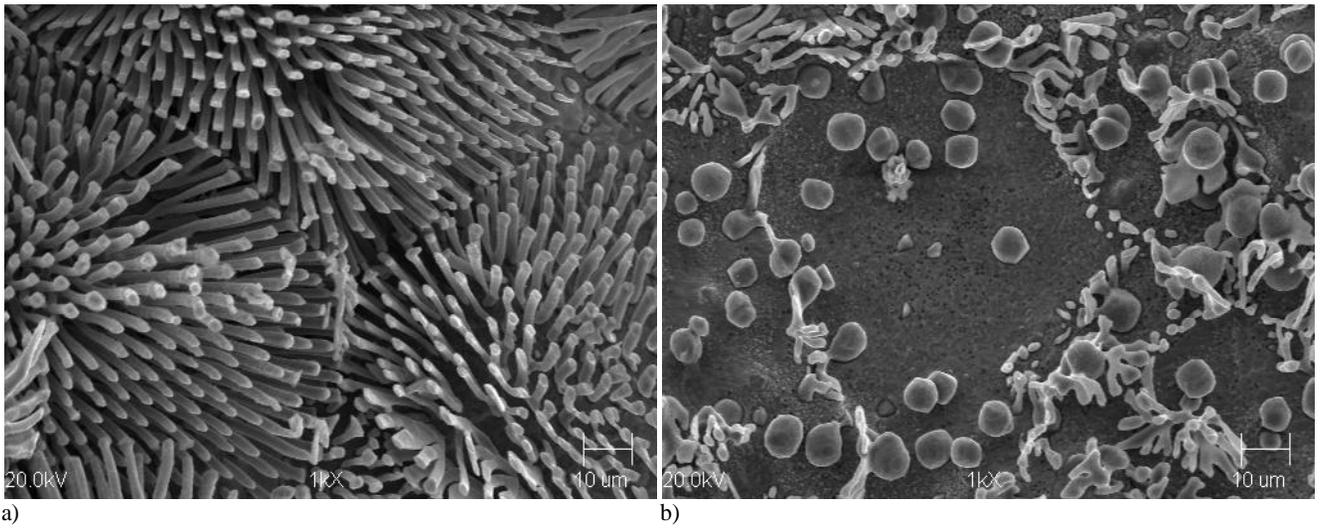
Fig. 3. Microstructure of alloy as-cast (a) and after the spheroidising treatment (b); deep etching with aqua regia (SEM)
