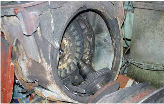
Figure 3. Condition of damaged main propulsion turbocharger rotor. Source based on ATSB (2006)
