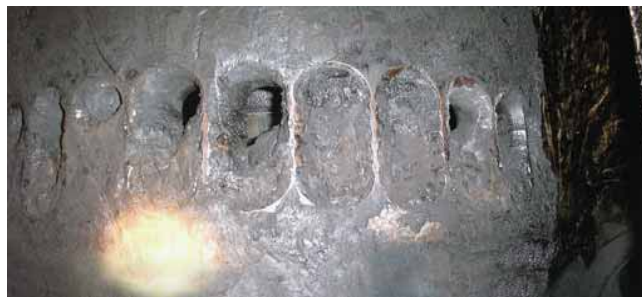
Figure 1. Condition of scavenge ports on Cylinder no. 1 of Main propulsion Engine Source based on ATSB (2006)
