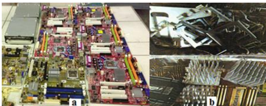
Fig. 1. PCBs of personal computer (a) and mounted parts (b)
