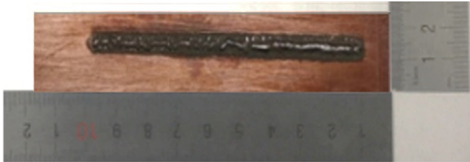
Fig. 3. Macro image of BCuP-5 coated on Ag plate using laser cladding process
