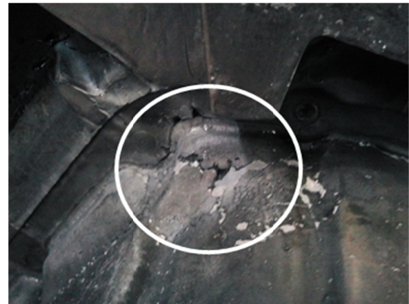
Fig. 3 Photograph of the damaged portion of the die
