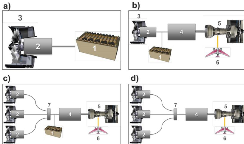
Fig. 2. Comparison of different types of architectures: a) full-electric propulsion system, b) parallel hybrid propulsion system, c) series hybrid, d) turboelectric. 1 – battery, 2 – electric motor, 3 – fan or propeller, 4 – generator, 5 – turbine engine, 6 – fuel tanks, 7 – power buss
