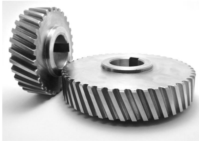
Fig. 6. Novikov gear pair, in which the presented method of axes distance error compensation was used
