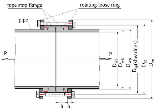
Fig. 1. Cross-section of a flanged joint
