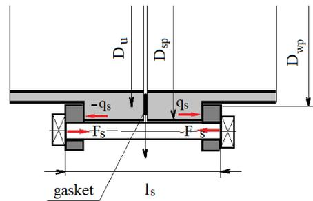
Fig. 2. Cross section of the connection with the marked loads of the rings  $F_s$  of the bolt pressure
