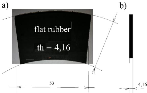
Fig. 8. View of flat rubber gasket sample (a) and its cross-section (b)
