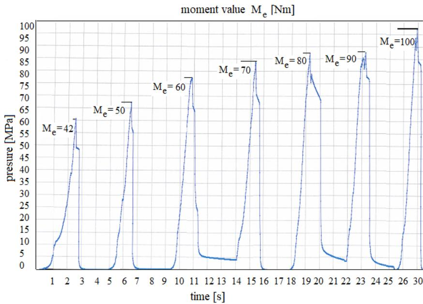
Fig. 15. Connection pressure test course
