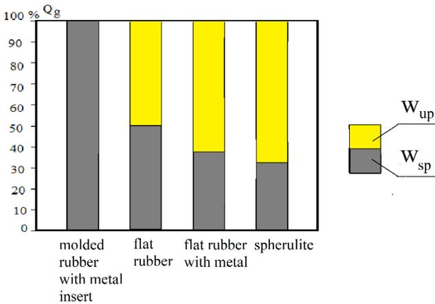
Fig. 12. Pressure load distribution of ring, including bolts  $q_s$  and gasket  $q_u$
