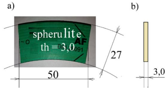
Fig. 10. View of a vertebralite gasket specimen (a) and its cross-section (b)
