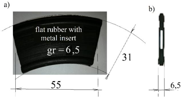
Fig. 7. Sample view of a shaped rubber gasket with a metal insert (a) and its cross-section (b)
