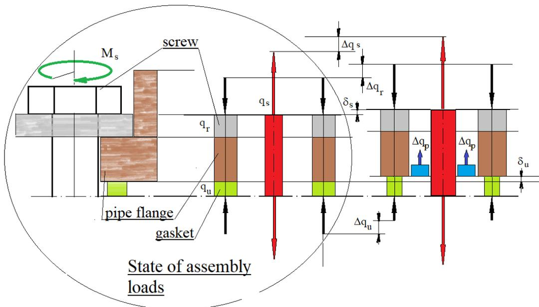
Fig. 5. Model of the elastic structure of the joint with the marked components of the loads from the pressure  $p$  and axial deformations of the elements
