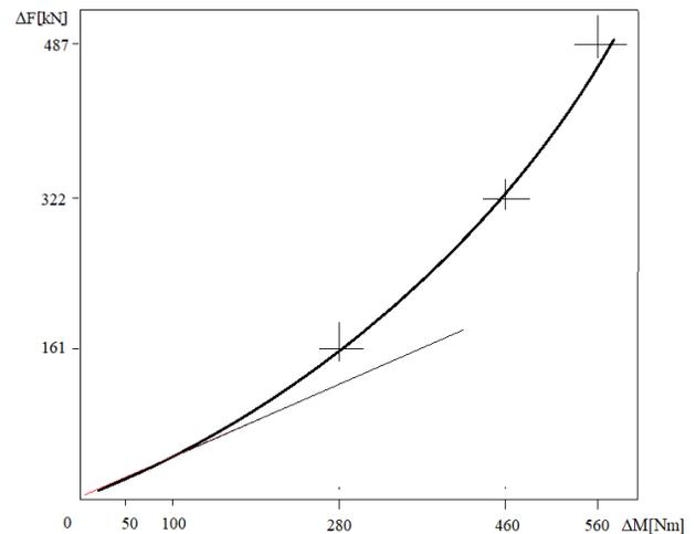
Fig. 4. Plot of bolt tension force versus tightening torque
