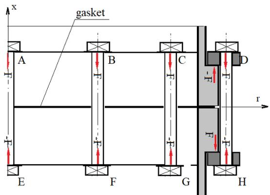
Fig. 3. Flange connection diagram for 12 connecting bolts
