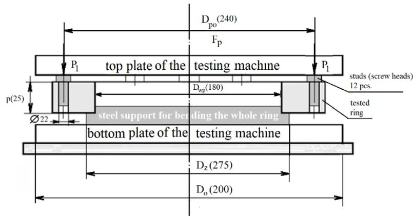
Fig. 13. Schematic of the test stand for ring stiffness, with the system of loads in the bend test
