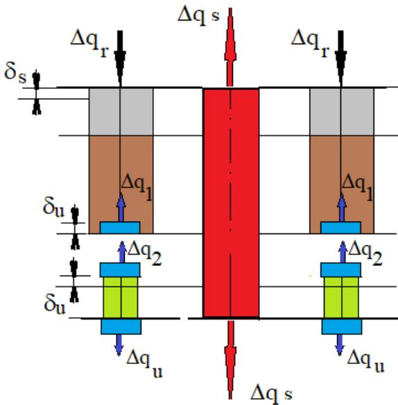
Fig. 6. Loads and deformations of joint components caused by change of pressure load by  $\Delta q_p$
