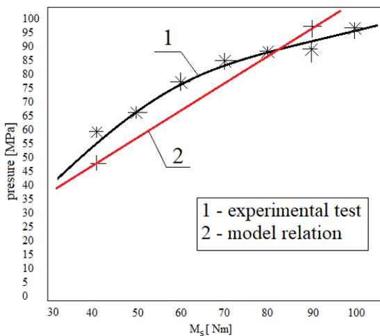
Fig. 16. Plots of leakage pressure on the assembly bolt tightening torque
