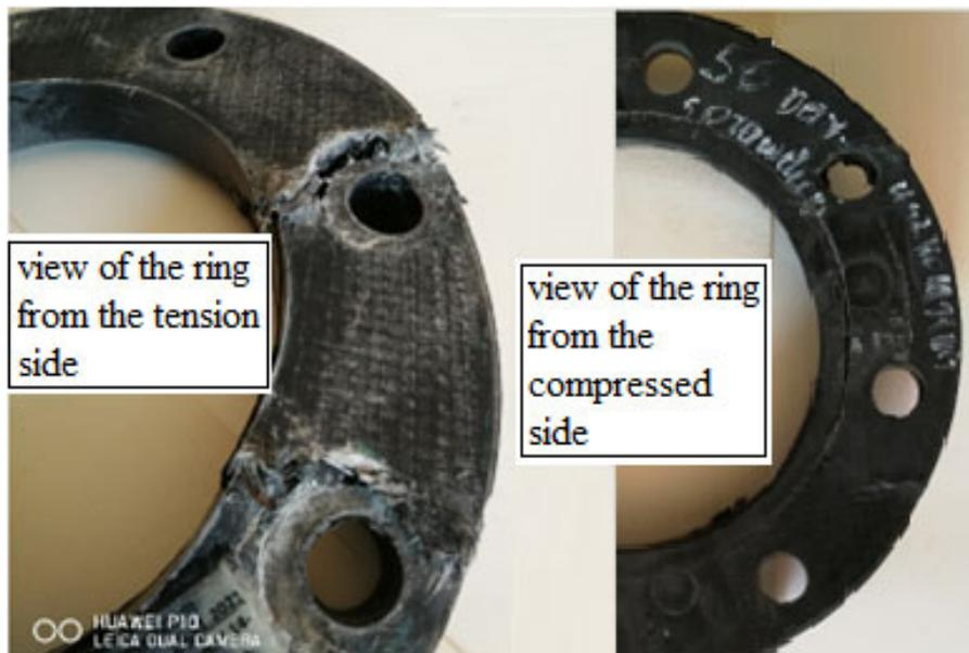
Fig. 17. View of the ring after the destructive test
