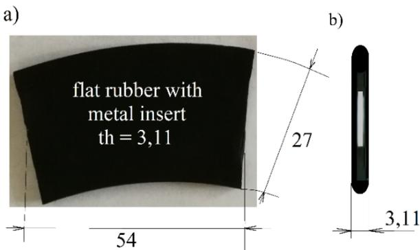
Fig. 9. Sample view of flat rubber gasket with metal insert (a) and its cross-section (b)
