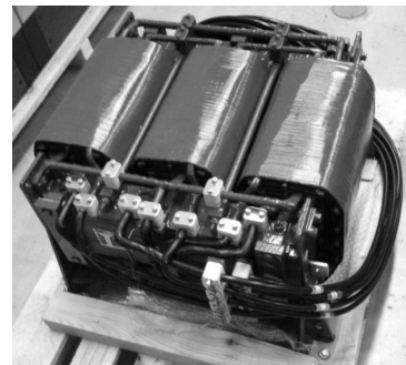
Fig. 3 Three-phase transformer with an additional magnetic core (increased leakage inductance)
