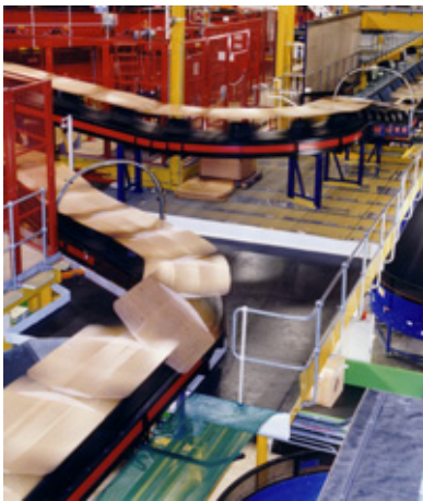
Figure 4. Luggage check and handling system built by Logan Teleflex
