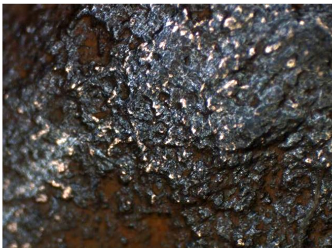
Fig. 7. Surface of copper rod, 50×
