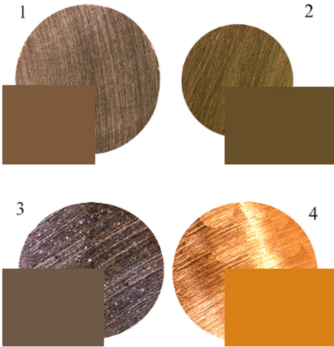
Fig. 10. Model alloys GST1-GST4. Cross-sections of model alloy samples, for archeological copper alloys with different content of intentional alloy additions as well as elements connected with their origin and technology: 1 – GST1 – CuSn11; 2-GST2 – CuSn8Pb1As1Sb1Fe2Ni1; 3 – GST3 – CuPb32As2Sb6Fe1Ni2; 4- GST4 – CuAg1Sb1As0.3
